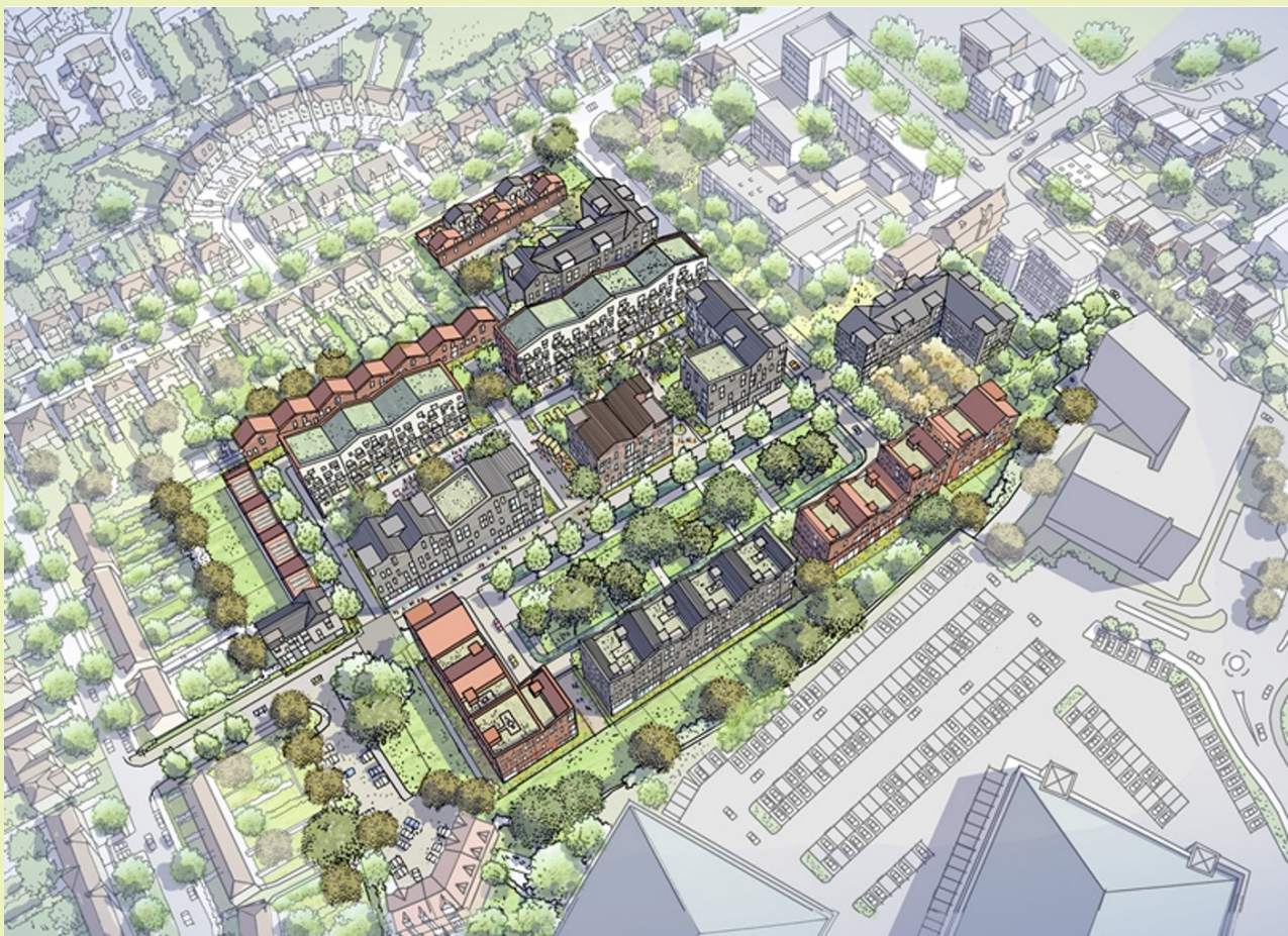
Grange Farm, South Harrow by Hawkins Brown shows how a new large-scale development can integrate with a range of contexts by modulating height and massing across the scheme. Height is stepped down for the north of the site, with new townhouses creating a gradual transition to areas of existing two-storey dwellings beyond and stepped up to the south through larger apartment blocks.
